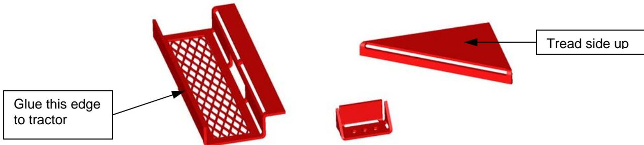
3. The steps are designed to overlay the existing cast ones, three on each side. For a more accurate model, the existing steps can be removed, leaving only small edges for the replacement to glue on. The back corner can then be trimmed to give an open look as shown below.
