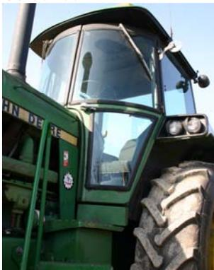
**Left:** Deere 4440 showing old style left wiper and door latch, mirror and antenna placement. Note door handle is to the left of the bottom window.
